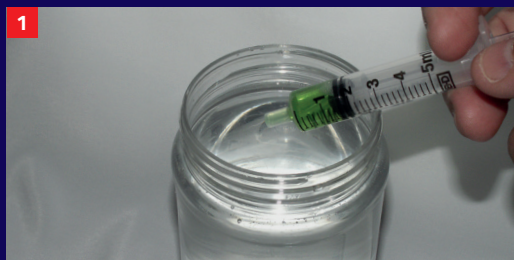
1 Class A foaming agent is added to the water at the proportioning rate recommended by the manufacturer.
