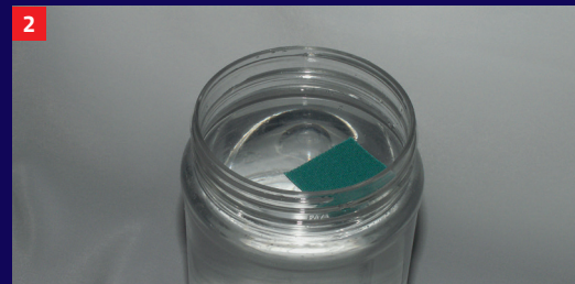
2 The pure water does not soak the swatch, the top of the swatch remains dry.
